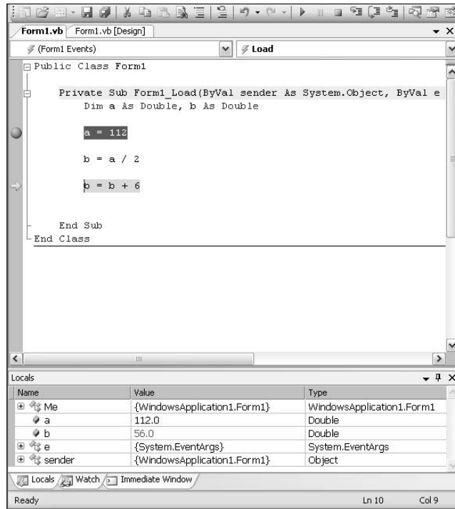
Figure 10-3: The Locals window displays the contents of all local variables in the currently executing procedure.
