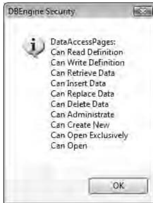
Figure 15-4: Every object type has a separate security container that you can validate.
