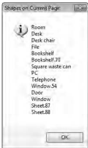
Figure BC2-3: Each shape on a page appears as part of that page's Shapes collection.
