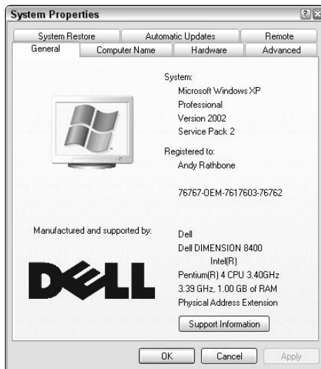
Figure 1-2: This PC runs Windows XP's Professional version on a 3.40 GHz Intel Pentium 4 CPU with 1GB of RAM.
