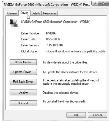
Figure 19-13: Click the Driver Details button in the Properties dialog box to view information about a part's drivers.
