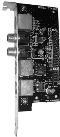
Figure 11-2: High-end sound cards often take up two slots by using a second card to add more connectors.
