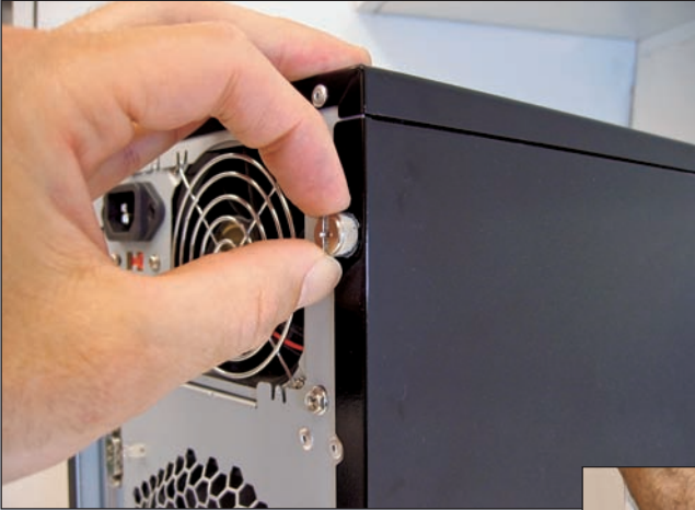
Color Plate 2: On other cases, you need to unscrew two thumb-screws.
