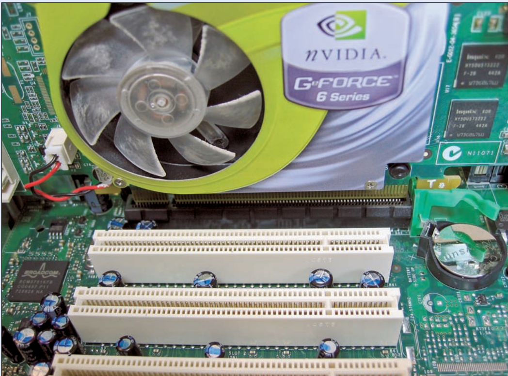
Color Plate 23: Push the card firmly into its slot. If you're installing a video card with a little fin, make sure the fin is held in place by the plastic holder. (The holder is green in this photo.)
