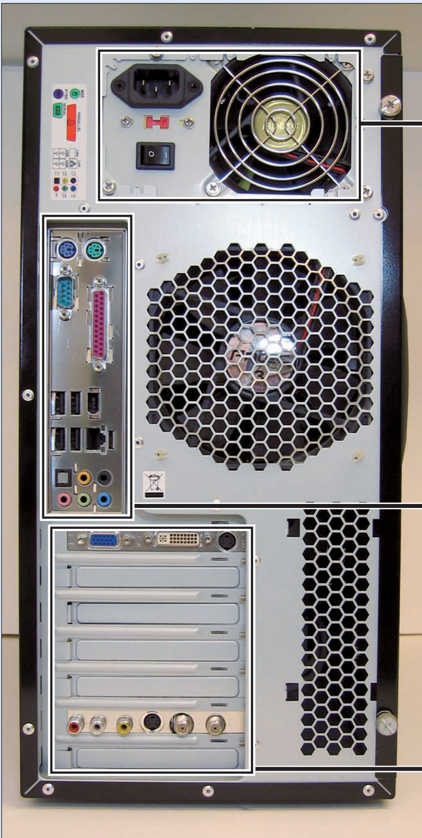
Color Plate 4: On the back of every PC, you see the power supply, the ports, and the slots.
