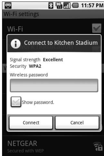
Figure 15-3: Enter your wireless password to continue connecting to this Wi-Fi network.
