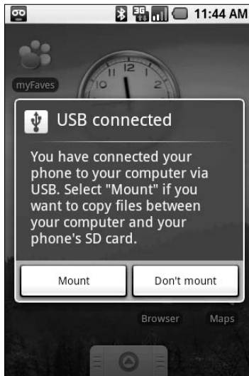
Figure 17-5: Confirm that you want to mount the memory card to your computer.
