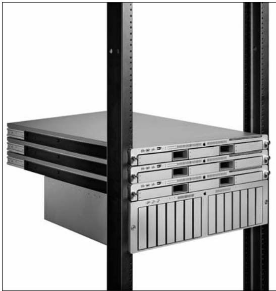
Figure 2-8: Three Xserves and a RAID mounted in a 19-inch rack.
