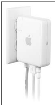
Figure 2-10: The AirPort Express, plugged in.
