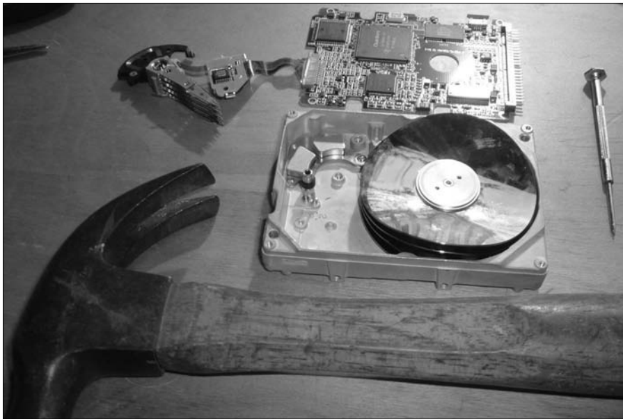
Figure 6-2: Dis- assembled hard drive with bent disks.
