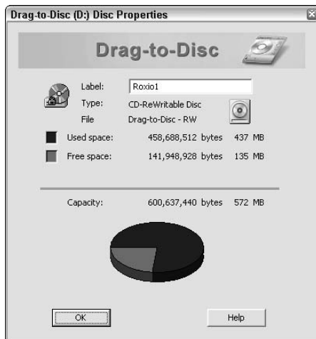
Figure 3-5: Use the Disc Properties dialog box to ascertain the type of disc (rewritable or non-rewritable) and the amount of free space.
