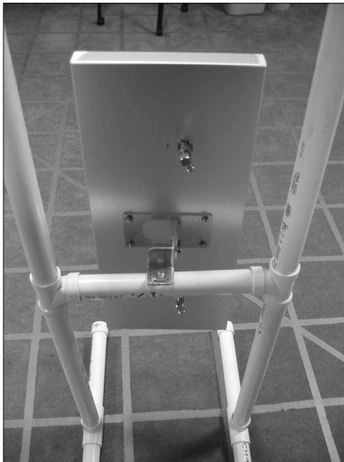
Figure 8-4: A home- made, freestand- ing PVC antenna rack.
