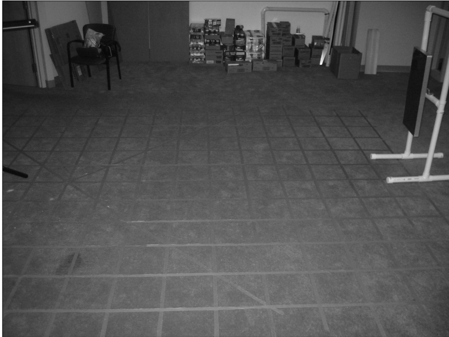
Figure 8-1: The floor grid pattern of your primary lab space helps you record accurate test results.
