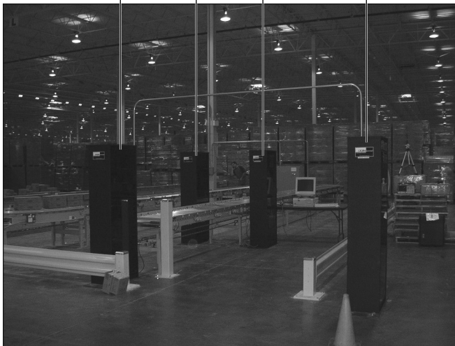
Figure 9-5: An “S” shaped conveyor with RFID tagging and verification stations.
