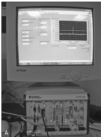
Figure 7-1: To test for AEN, use a spectrum analyzer and monitor (A) and a \frac{1}{2} -wavelength dipole antenna mounted to a tripod and grounding plane (B).
