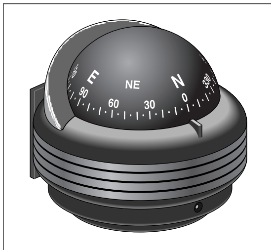
Figure 10-1: A compass shows your course in alignment with the center mark, called the lubber line.
