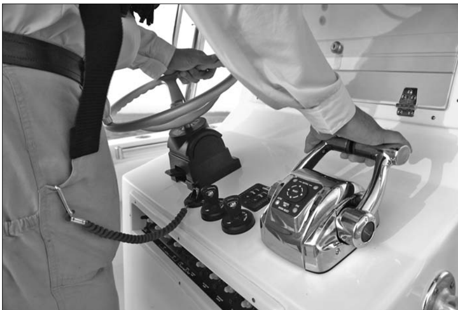
Figure 7-1: The kill switch needs to be connected at the ignition and to the captain.
