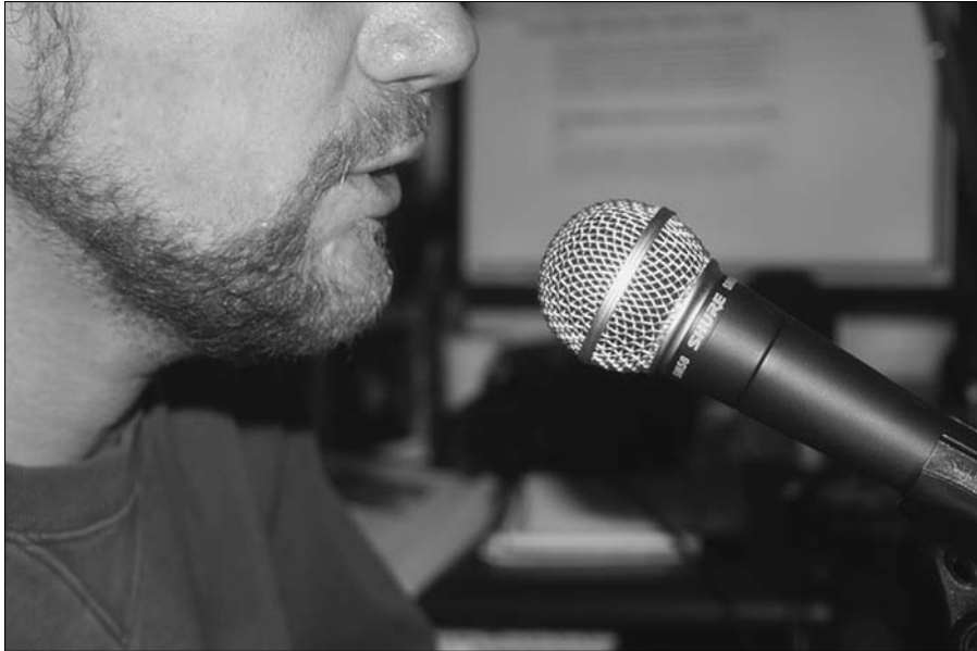
Figure 6-2: Set your microphone at a comfortable distance, close enough to overpower ambient noise, but far enough to avoid microphone contact.
