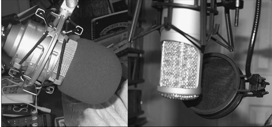
Figure 2-9: Wind-screens (left) and pop filters (right) help you control unwanted noise and percussive consonants (such as P and B ) during recording.
