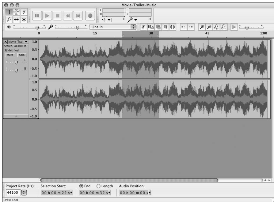
Figure 7-3: With the Selection tool, click and drag across the unwanted content in the timeline.
