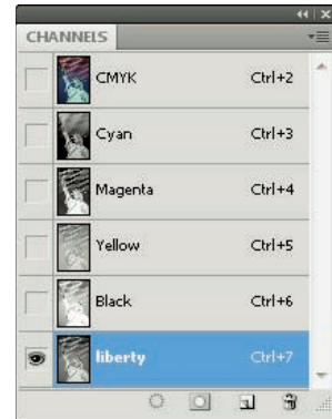
Figure 1-4: You can duplicate channels for masking, as well as for backup purposes.
