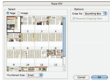
Figure 3-5: Use the Place command when importing a page from a multipaged PDF into an existing file.
