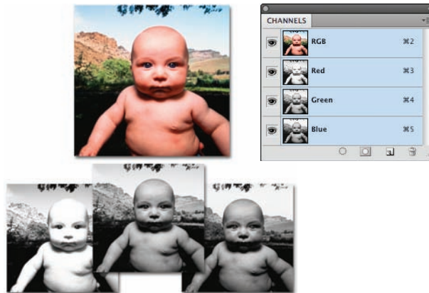
Figure 1-1: A color image is composed of 8-bit grayscale images referred to as channels.
