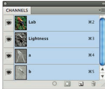
Figure 2-5: Lab Color mode is the preferred editing mode for color experts because it’s device-independent.
