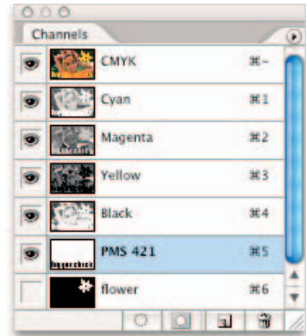
Figure 1-1: A color image is composed of 8-bit grayscale images referred to as channels.
