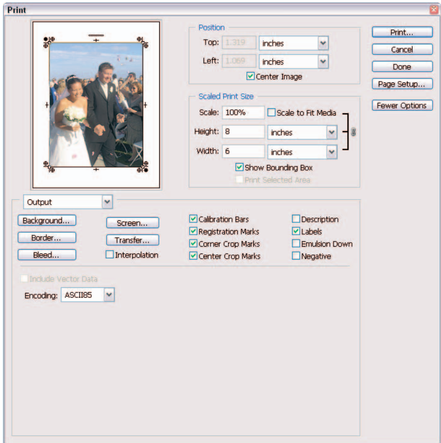
Figure 1-3: When printing color separations, be sure and check the necessary options in the Output section of the Print with Preview dialog box.
