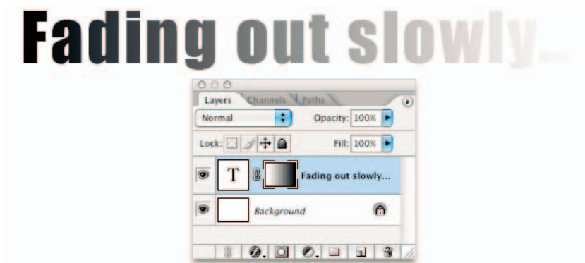
Figure 3-14: Fade your text gradually by applying a gradient on a layer mask.
