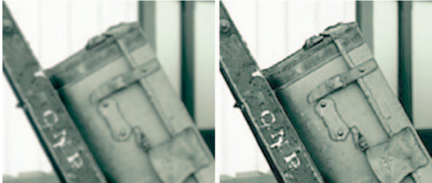
Figure 1-3: Sharpening an image boosts the contrast of neighboring pixels and gives the illusion of improved focus.
