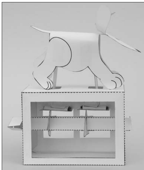
Figure 10-22: The pushrods attach to the cam followers.
