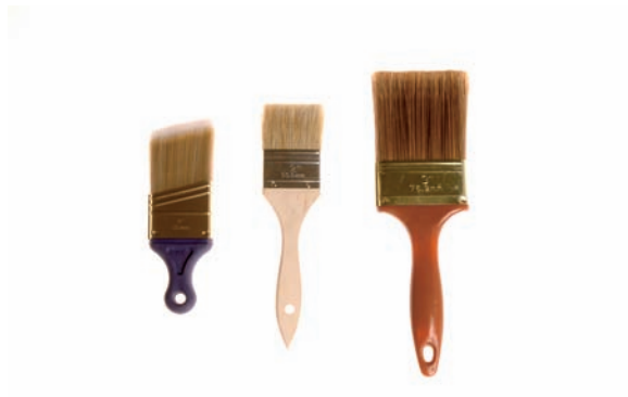
Figure 1-5: A 2-inch angled sash brush, a small chip brush, and a 3-inch flat sash brush.
