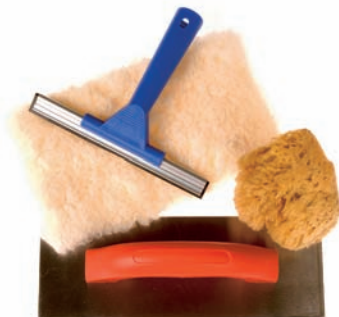
Figure 1-12: A sheepskin pad, a sea sponge, a shower squeegee, and a large steel trowel.
