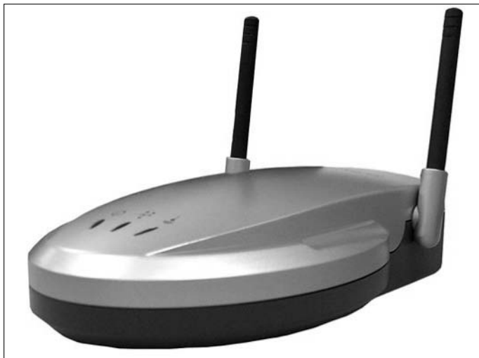
Figure 3-1: A typical WAP for your LAN. (Try to keep a straight face when you say that.)
