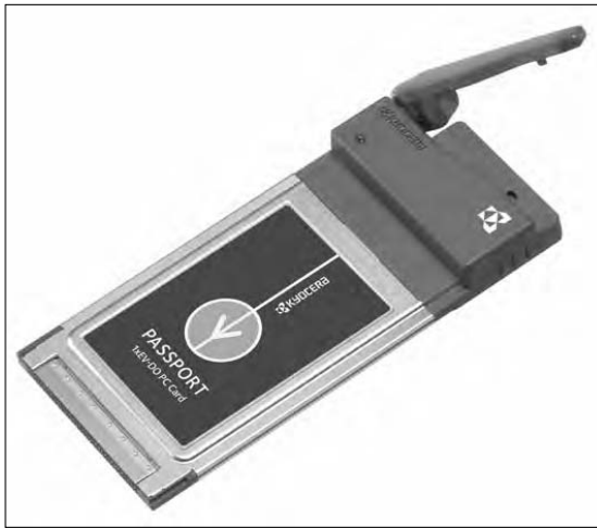
Figure 7-1: The Kyocera Passport KP650 cellular data card comes equipped with a sensitive adjustable antenna that folds neatly away when not needed.
