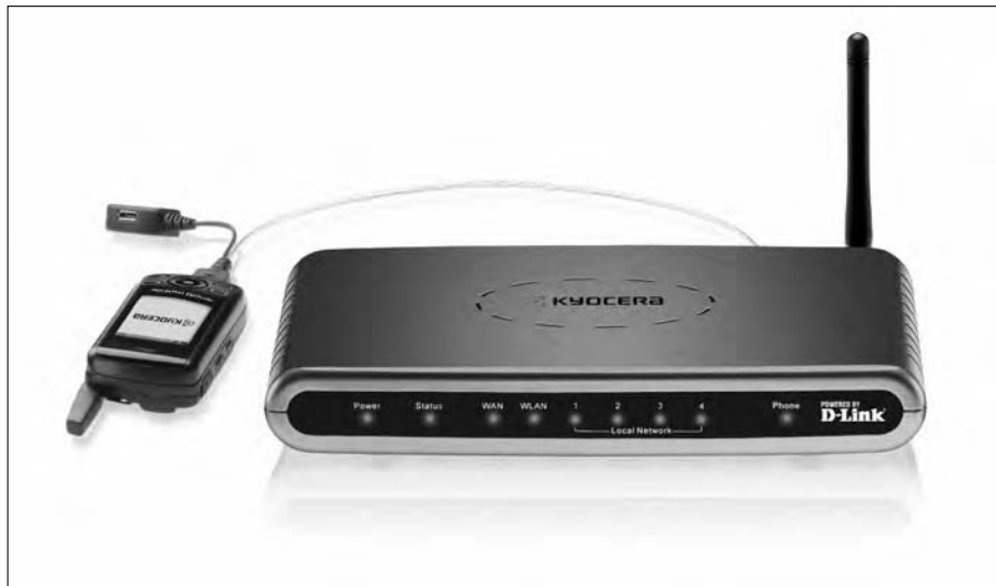
Figure 7-4: The Kyocera KR1 Mobile Router, shown using a cellphone as con- nection medium.
