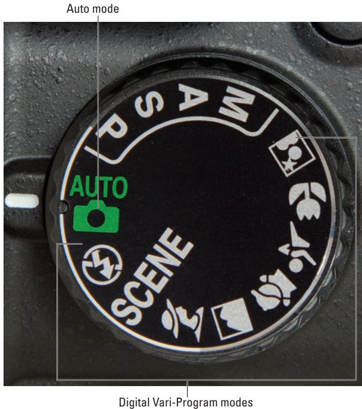
Figure 2-7: You can select from eight fully automatic, point-and-shoot photography modes, and a Scene mode.
