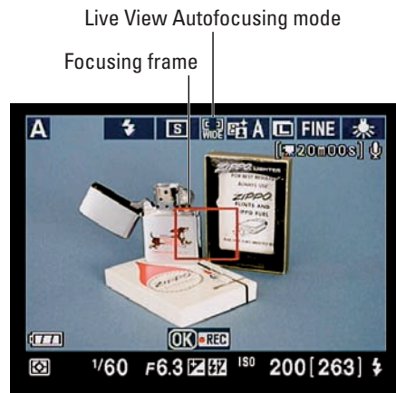
Figure 6-9: In the default Live View display mode, an icon representing the focusing mode appears here.
