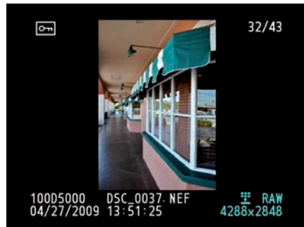
Figure 4-25: Press the AE-L/AF-L button to prevent accidental deletion of the selected image.
