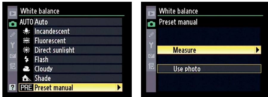
Figure 6-22: Select these options to set white balance by measuring a white or gray card.
