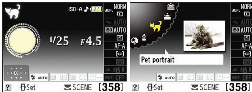
Figure 2-12: After setting the Mode dial to Scene, rotate the Command dial to select the type of picture you want to capture.
