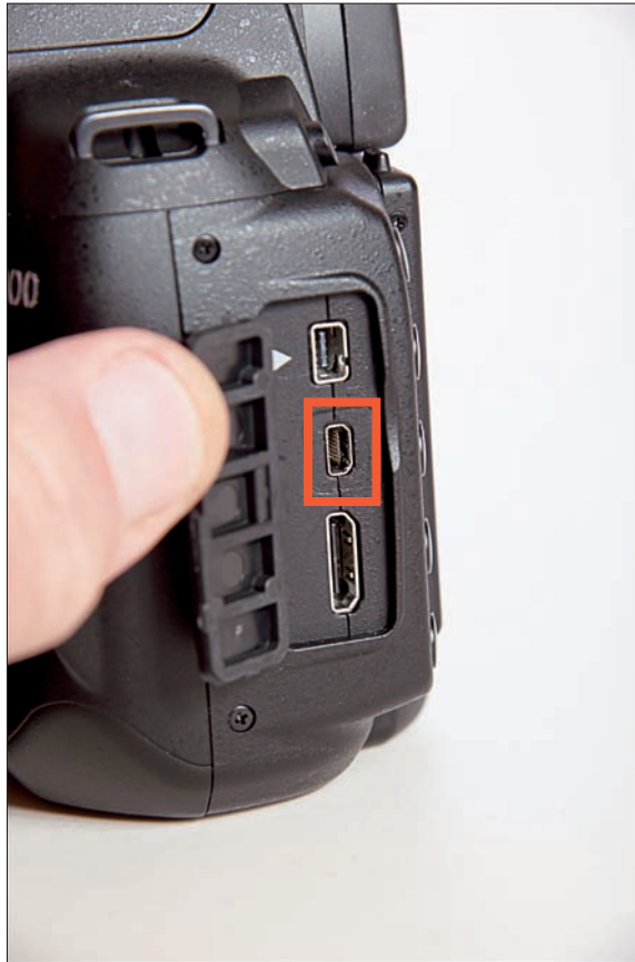
Figure 8-3: The USB slot is hidden under the rubber door on the left side of the camera.
