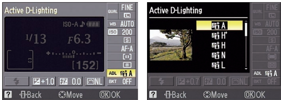
Figure 5-26: You can change the Active D-Lighting setting easily via the Quick Settings screen.
