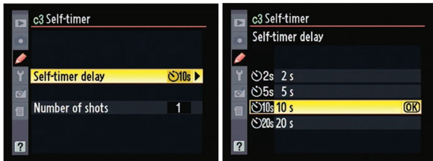
Figure 2-13: You can adjust the self-timer capture delay via the Custom Setting menu.
