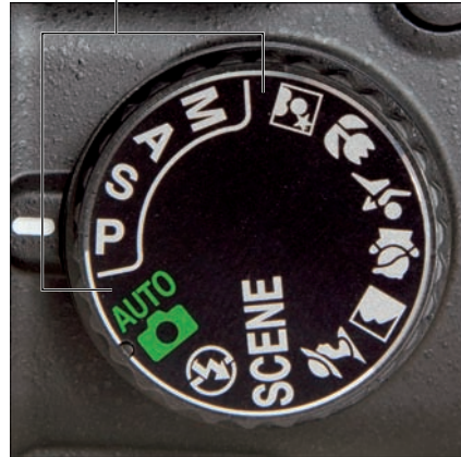
Figure 5-8: You can control exposure and certain other picture properties fully only in P, S, A, or M mode.
