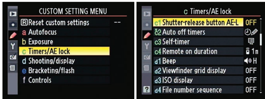
Figure 1-20: Highlight a submenu and press OK again to access the available settings.
