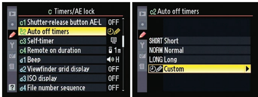
Figure 1-21: Visit the Timers/AE Lock submenu to adjust the timing of automatic monitor, viewfinder, and metering shut-off.
