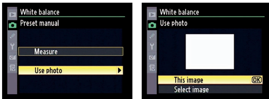
Figure 6-24: You can create a white balance preset based on an existing photo.
