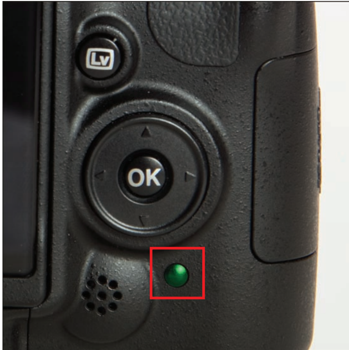
Figure 2-4: The memory card access lamp lights while the camera sends the picture data to the card.
