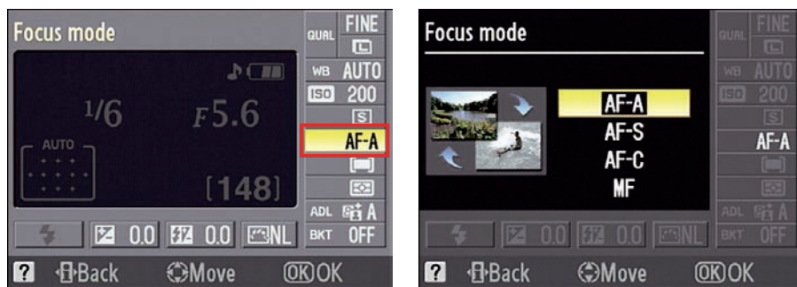
Figure 6-8: The Focus mode determines whether the autofocus system locks focus when you press the shutter button halfway.
