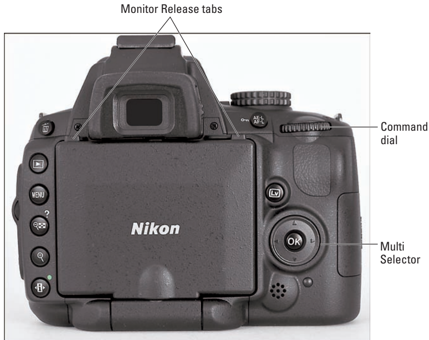
Figure 1-8: You use the Multi Selector to navigate menus and access certain other camera options.
