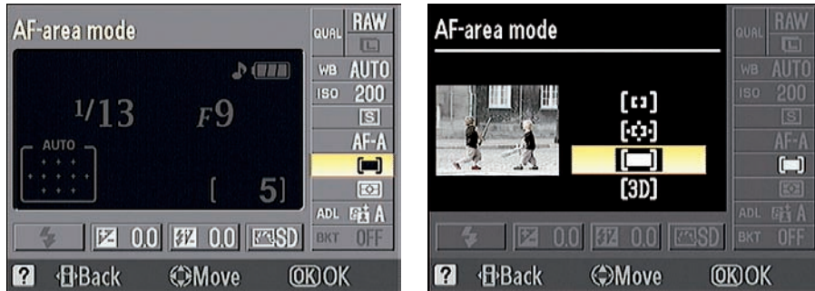
Figure 6-5: The fastest way to adjust the AF-area mode is through the Quick Settings screen.
