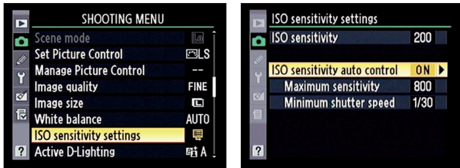
Figure 5-17: You can also set ISO and access additional ISO options through the Shooting menu.
