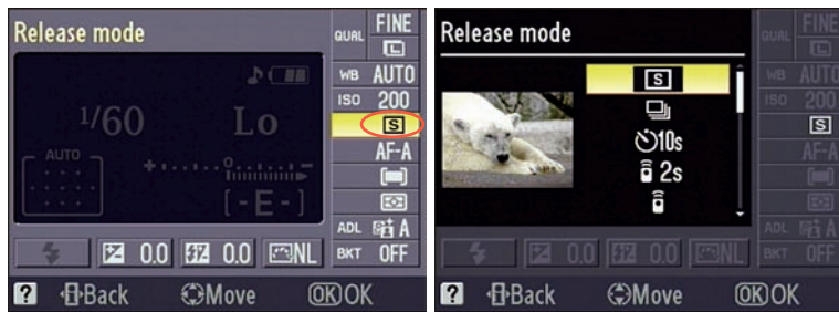
Figure 2-14: You can check the current Release mode in the Shooting Information display.
