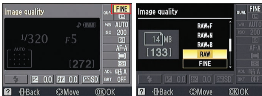
Figure 3-7: You can use the Quick Settings screen to change the Image Size and Quality settings.
