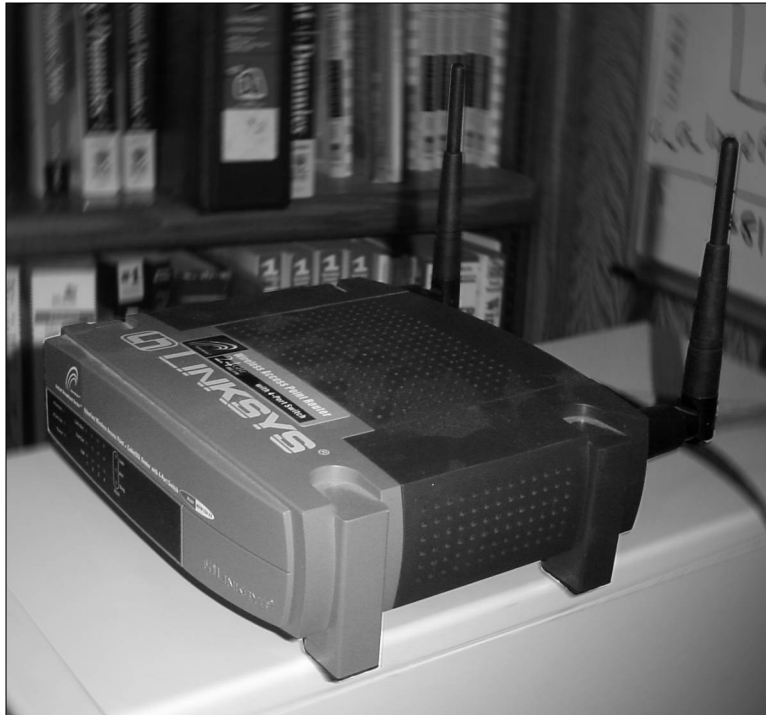
Figure 1-5: A Linksys BEFW11S4 wireless access point router.
