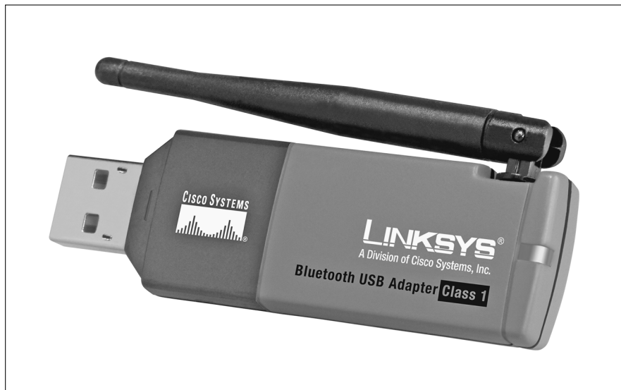
Figure 5-1: A typical USB Bluetooth adapter.
