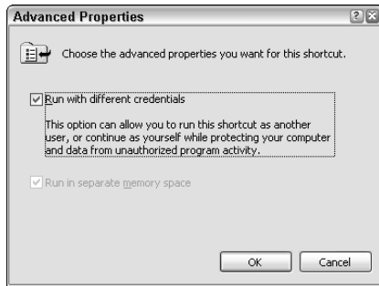
Figure 6-7: Setting the RunAs feature for a desktop shortcut.
