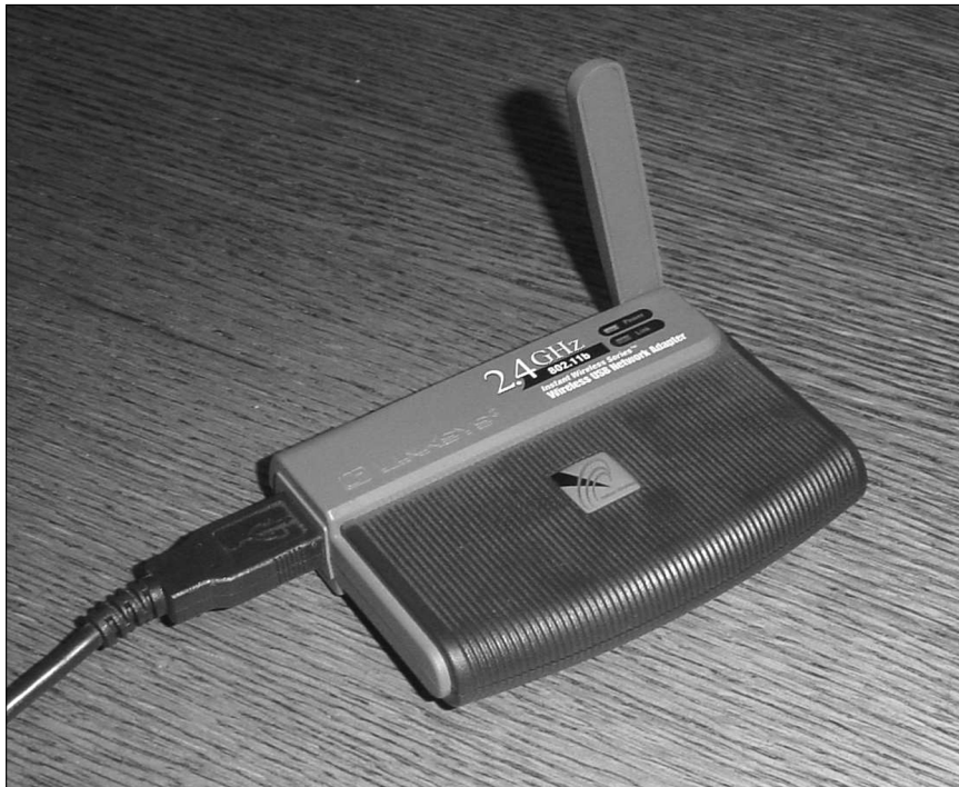
Figure 1-3: A Linksys WUSB11 USB 802.11b Wireless networking adapter.
