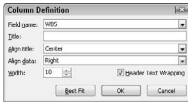
Figure 3-2: Use this dialog box to insert a column in the table that displays WBS codes.
