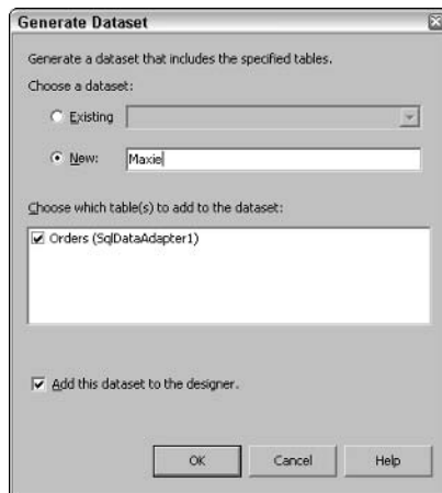
Figure 2-4: Use this dialog to name a new DataSet (or modify an existing one).
