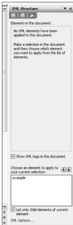
Figure 6-5: After you add a schema to a Word document, an XML Structure task bar appears.
