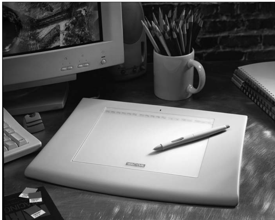
Figure 3-13: This Wacom pen and tablet set is easier to draw with than a mouse and enables you to easily vary the brush width as you draw.
