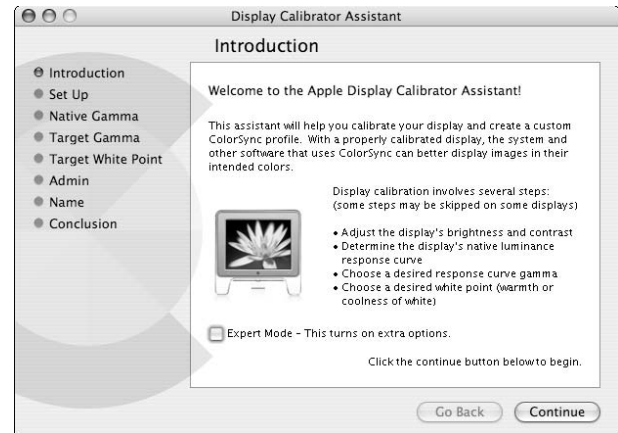
• Figure 8-5: Use the Display Calibrator Assistant to create your monitor's color profile.
