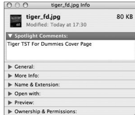
• Figure 20-11: Add comments to a file by using the Get Info panel.
