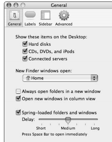
• Figure 9-8: Use the Finder's preferences panel to set column view as the default.
