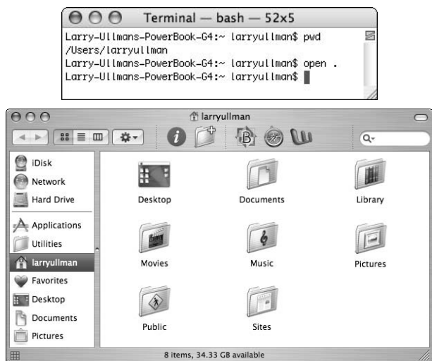
• Figure 56-15: The open command makes quick transitions between the Terminal and the Finder.
