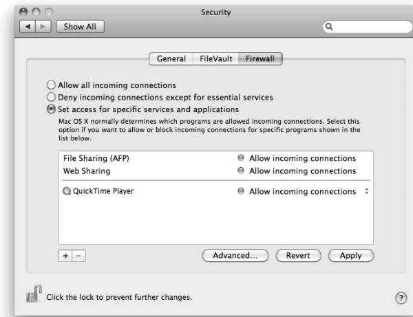
Figure 17-4: I enabled File Sharing and Web Sharing in the Sharing System Preference pane and opened the firewall for QuickTime Player.
