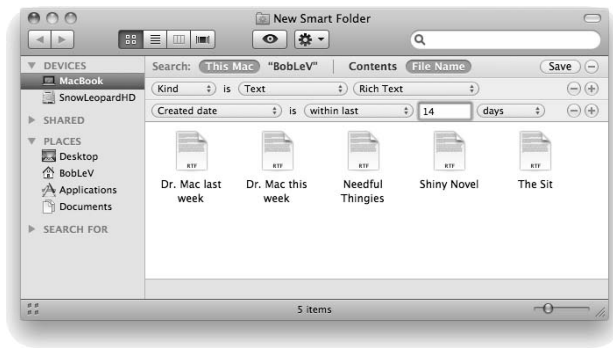
Figure 6-16: A Smart Folder that gathers only Rich Text files created in the past two weeks.
