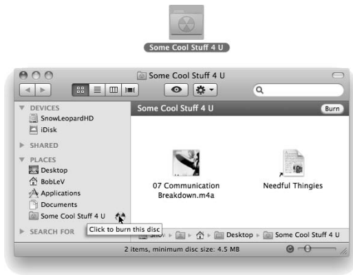
Figure 7-6: Clicking the burn icon to burn the items in a Burn Folder to disc.
