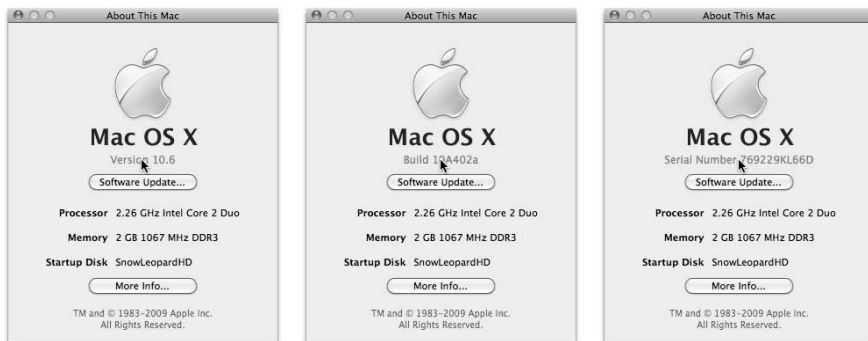
Figure 2-11: Click the Version, build, or serial number to cycle through these three informative items in this window.
