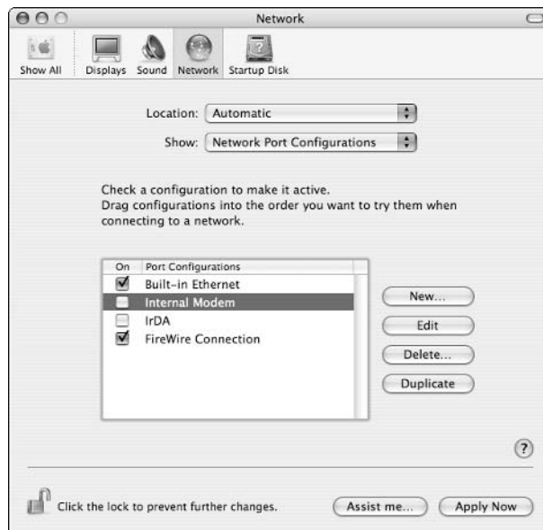
• Figure 39-9: Check your active network ports before sharing a connection.
