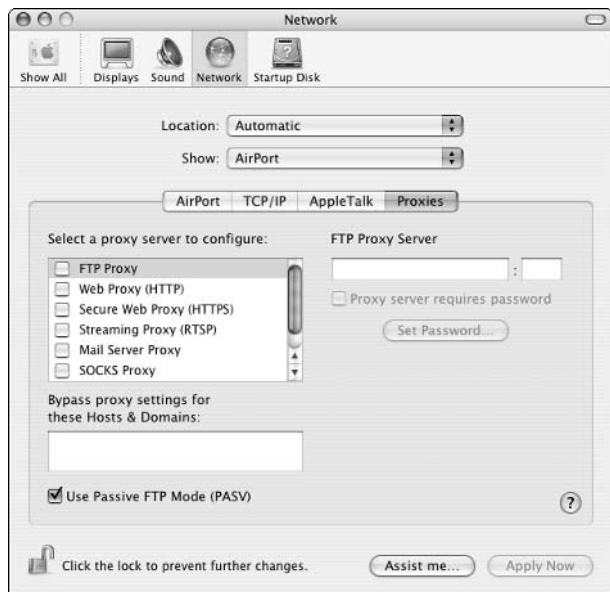
• Figure 40-3: Enable PASV to use FTP when your Mac is behind a firewall.
