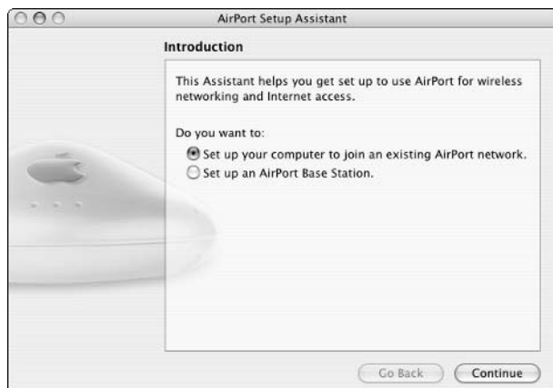
• Figure 37-1: Use the AirPort Setup Assistant to connect to an existing network or set up a new one.
