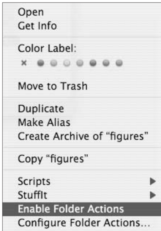
• Figure 12-5: You must enable Folder Actions for the system before you can use them.
