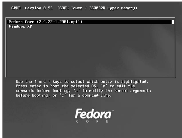
Figure 2-7: Dual-boot startup screen for a system with Fedora Core 1 and Windows XP installed.
