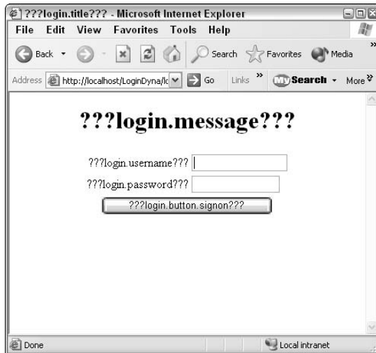
Figure 7-1: A message resource is missing, so the application displays lots of question marks.
