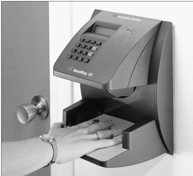
Figure 6-7: A biometric hand reader and PIN- pad device.
