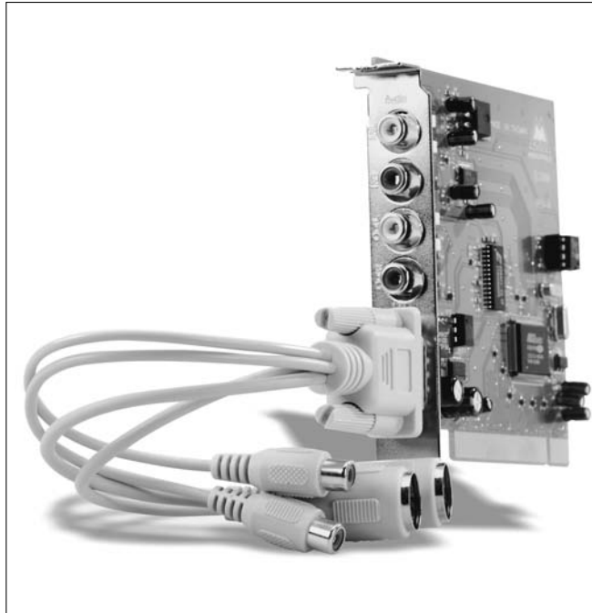
Figure 2-2: PCI interfaces often come with analog connectors run from the computer.
