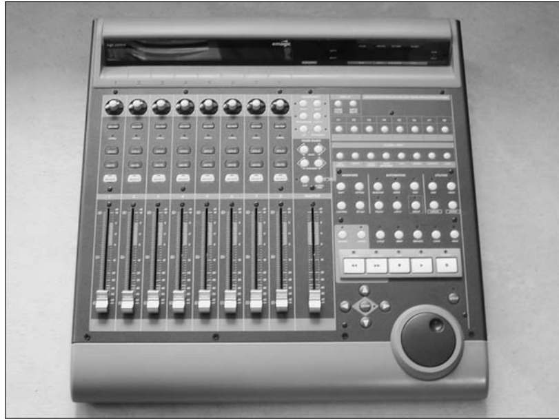
Figure 4-4: A computer control surface acts like a digital mixer for a computer-based system.
