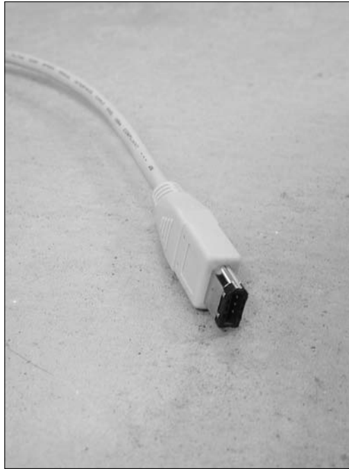
Figure 3-9: FireWire is a high-speed data- transfer protocol.
