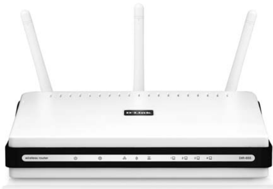
Figure 3-6: A wireless network router, shown here, has at least one antenna; a wired router has none.
