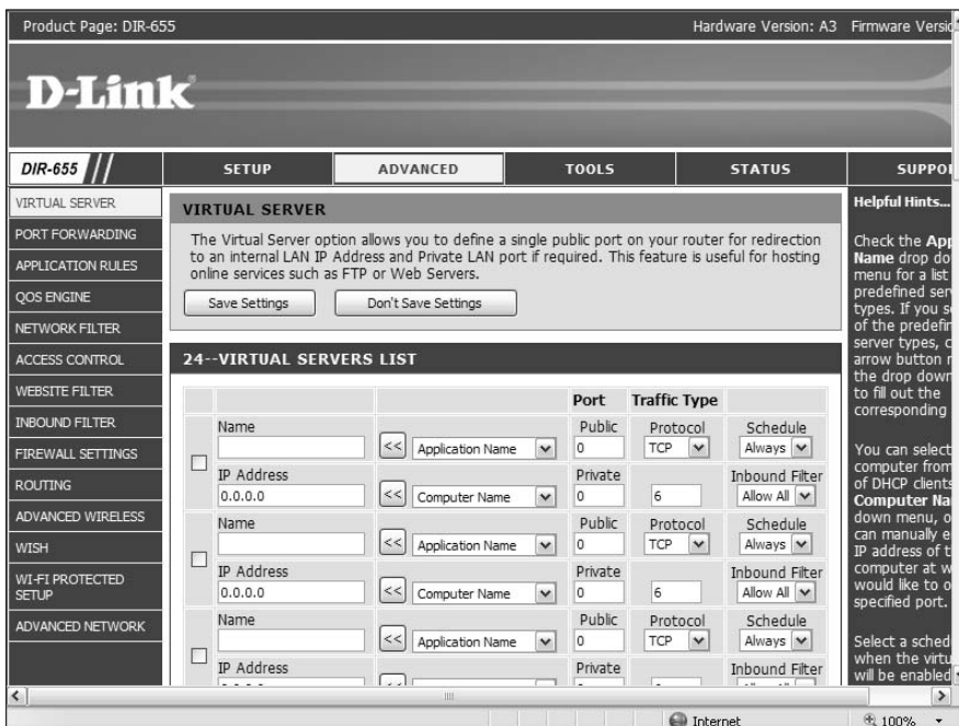
Figure 8-9: Virtual server settings of a wireless router.
