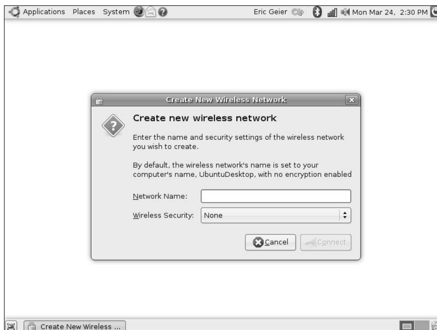
Figure 4-11: Creating a wireless ad hoc network in Ubuntu.
