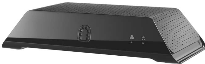
Figure 3-6: The Slingbox that you connect to your cable or audio/video source at home.
