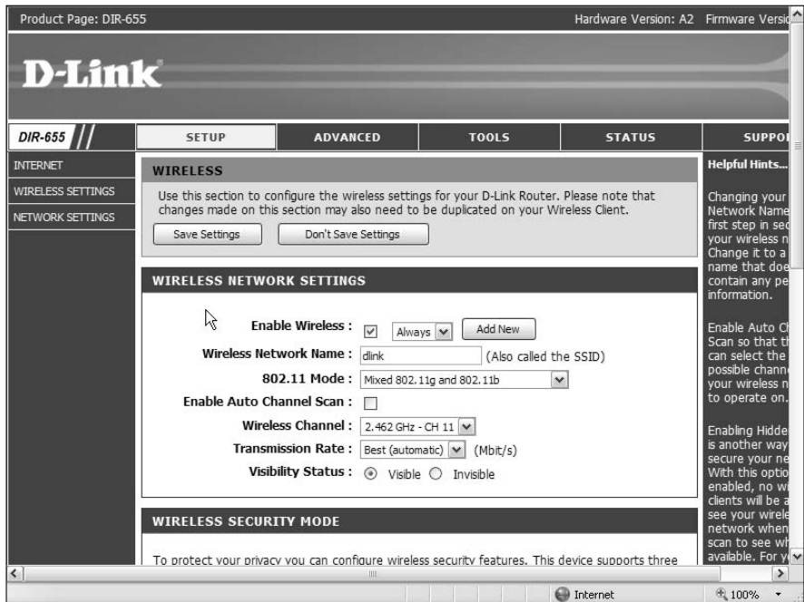
Figure 4-4: Wireless settings on a wireless router.
