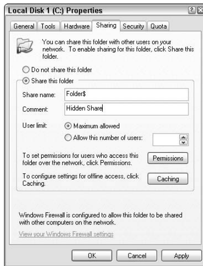
Figure 6-7: Creating a hidden share by appending a dollar sign to the Share Name.
