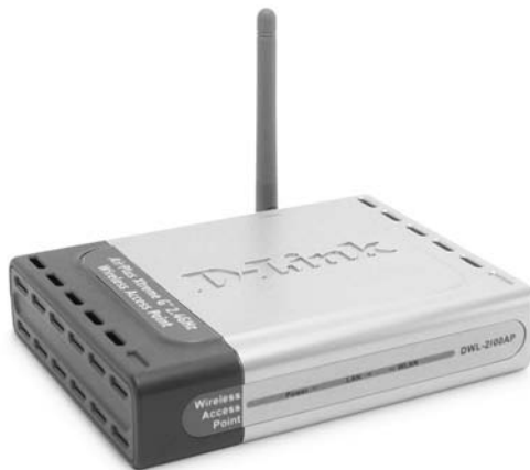
Figure 7-14: Example of an access point.
