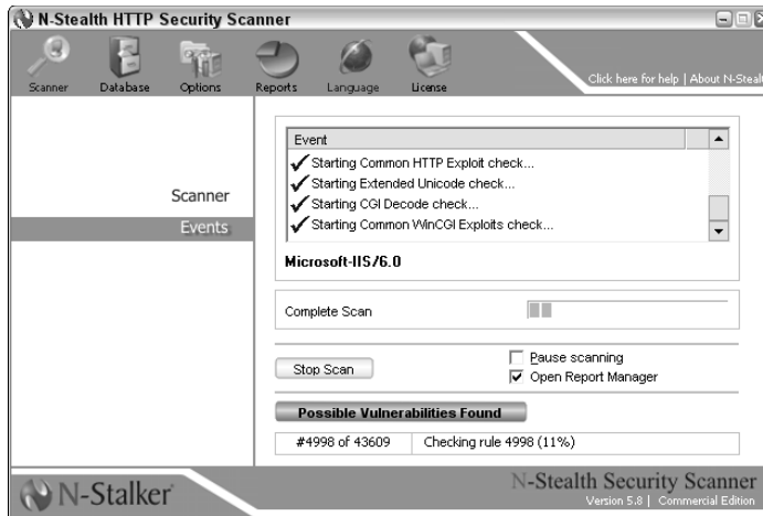
Figure 15-13: Using N-Stealth HTTP Security Scanner to check a wide range of basic Web application vulnera- bilities.
