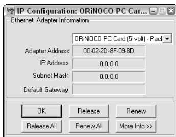
Figure 17-1: Using wntipcfg to release IP addresses.
