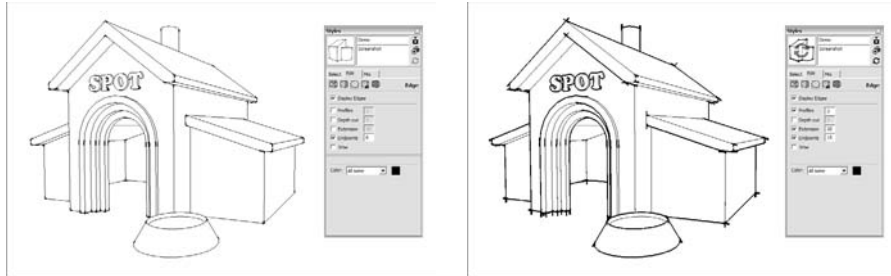
Figure 8-5: Endpoints give your model more visual impact. Used with Extension and Profiles or Depth Cue, they look even better.
