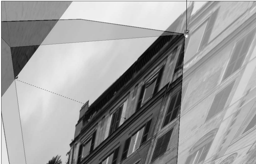
Figure 7-6: Drag the pin you just placed to the corresponding corner of the face you're working on.
