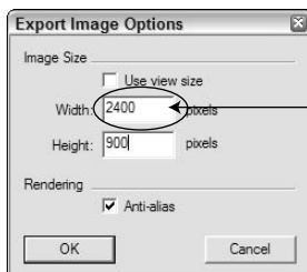
Figure 13-6: To figure out how many pixels you need to export, multiply the resolution by the physical size.
