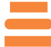
Figure 3-4: These lines were all drawn 88 pixels long, but the bottom two lines have round and square caps, so they're longer.
