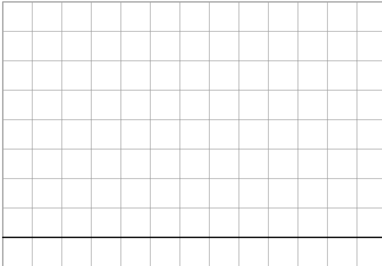
Figure 13-7: Adjust the Vertical Position knob so that the beam sits on the bottom of the grid.
