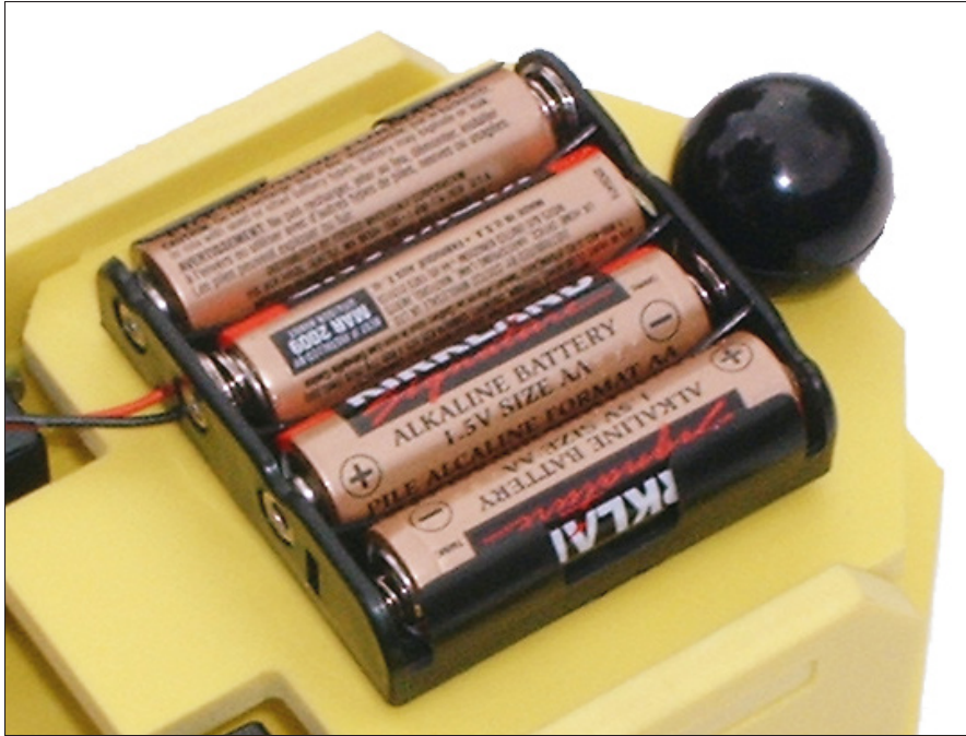
Figure 8-4: Four 1.5 volt batteries in a battery holder produce about 6 volts across the red and black leads.
