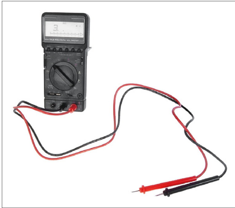
Figure 12-1: Multimeters measure voltage, resistance, current, and continuity.
