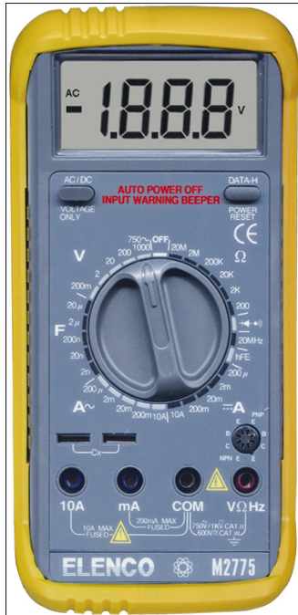
Figure 9-2: Multimeters measure voltages, resistance, and current.
