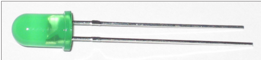
Figure 6-9: The shorter lead of a typical single-color LED is attached to the cathode.
