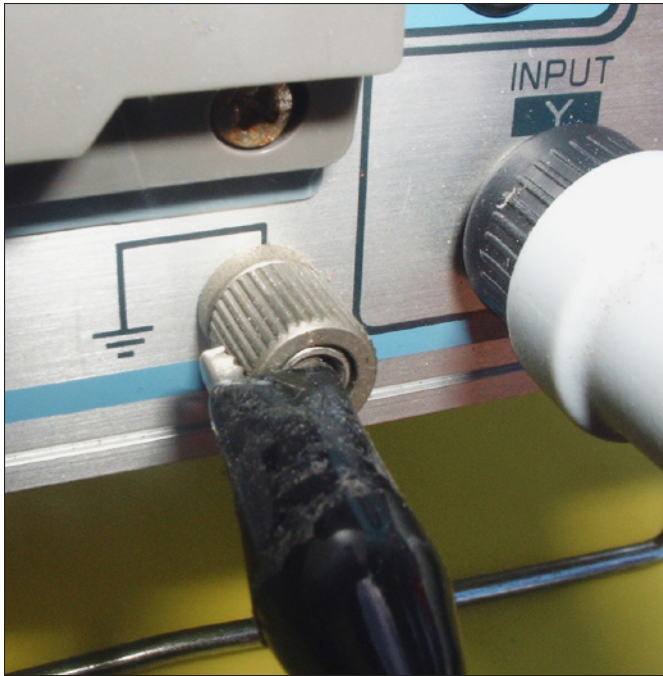
Figure 13-6: Connect the ground of the probe to the ground connec- tion on the scope.
