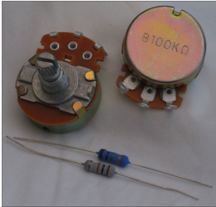
Figure 3-3: Color-coded bands denote the value of a fixed resistor; potentiometers are usually stamped with their highest resistance value.
