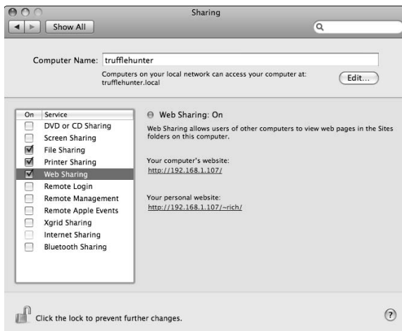
Figure 1-3: Turning on the Apache server.
