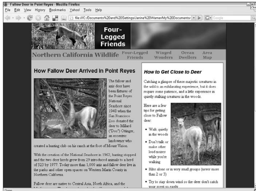
Figure 6-4: This page was designed using CSS to position the images and <div> tags to create the two-column layout and to wrap text around each image.
