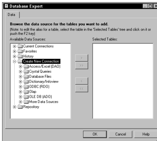
Figure 3-1: The Database Expert dialog box shows possible locations for the database you want.
