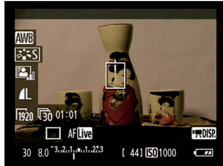
Figure 5-12: Setting exposure manually.
