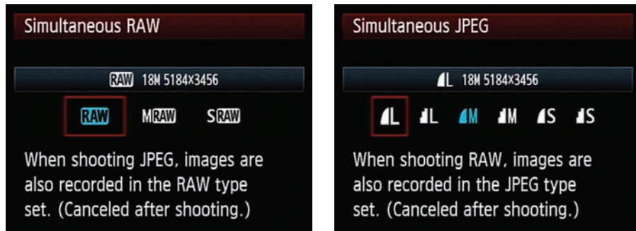
Figure 3-3: Choosing the RAW size and JPEG size as well as quality options for the RAW+JPEG button.
