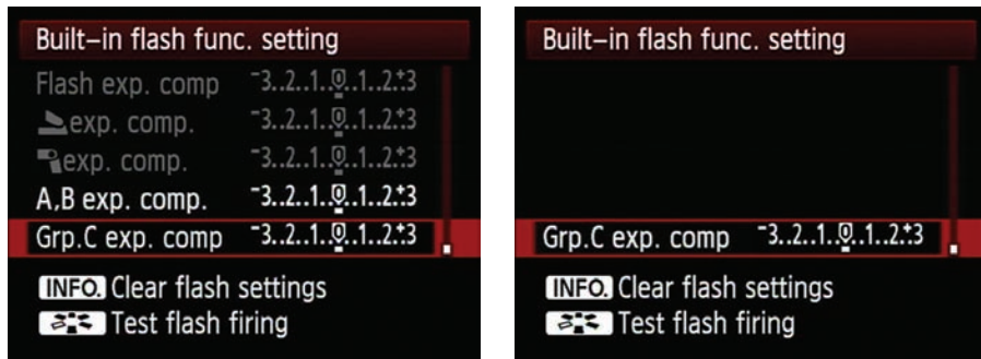
Figure 7-49: Setting Group C exposure compensation.
