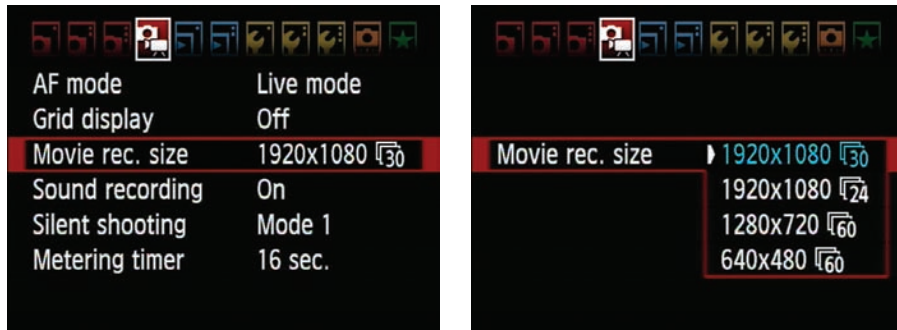
Figure 5-14: Changing video dimensions and frame rate.
