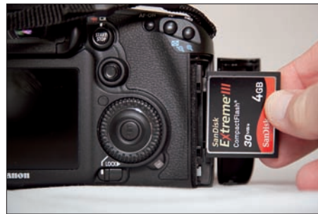
Figure 1-12: Inserting a CF card.
