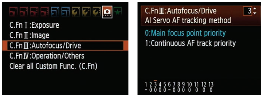
Figure 8-10: Changing the AI Servo autofocus mode tracking option.
