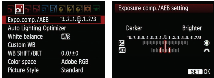
Figure 6-18: Setting automatic exposure bracketing.
