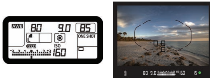
Figure 6-3: You can shift programmed exposure.
