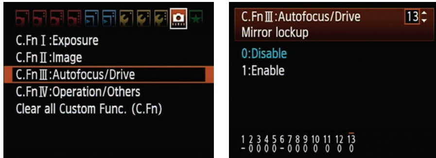
Figure 8-12: Enabling Mirror Lockup.
