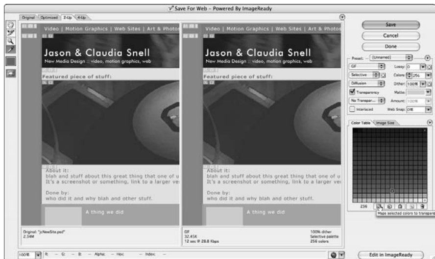
Figure 7-14: Click the Map Selected Colors to Transparent button to make a color disappear.
