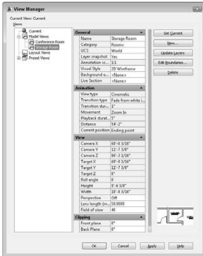
Figure 3-10: The View Manager dialog box is used to create and organize named views.
