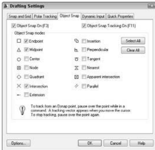
Figure 7-10: Snap to it . . . set running object snaps in the Drafting Settings dialog box.
