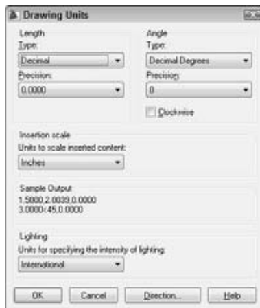
Figure 6-1: Format the display of drawing units in the Drawing Units dialog box.
