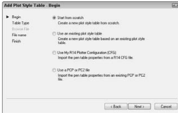
Figure 3-4: You use the Add Plot Style Table Wizard to create a plot style.
