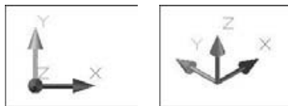
Figure 2-5: UCS icon displayed in model space with one of the 3D visual styles.
