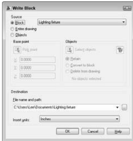
Figure 1-3: The Write Block dialog box is used to export a block definition.
