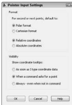
Figure 7-5: Controlling the format used for the second and next point when using dynamic input.
