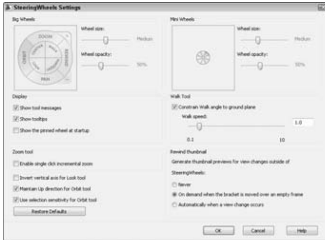
Figure 3-9: Changing the appearance and behavior of SteeringWheels with the SteeringWheels Settings dialog box.
