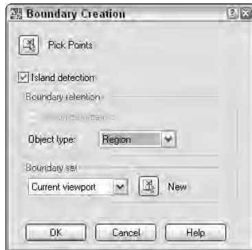
Figure 6-8: The Boundary Creation dialog box allows you to create regions based on loops.
