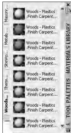
Figure 17-7: The Tool Palettes Window with the Materials Library tool palette group displayed.
