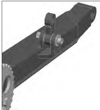
Figure 7-7: The com- pleted connection and align- ment of the transfer link.
