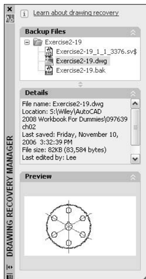
Figure 2-4: The Drawing Recovery Manager palette allows you to open files related to a drawing after a recent crash.
