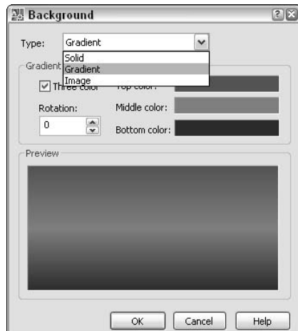
Figure 5-13: The Background dialog box allows you to assign a solid color, a gradient color, or an image.
