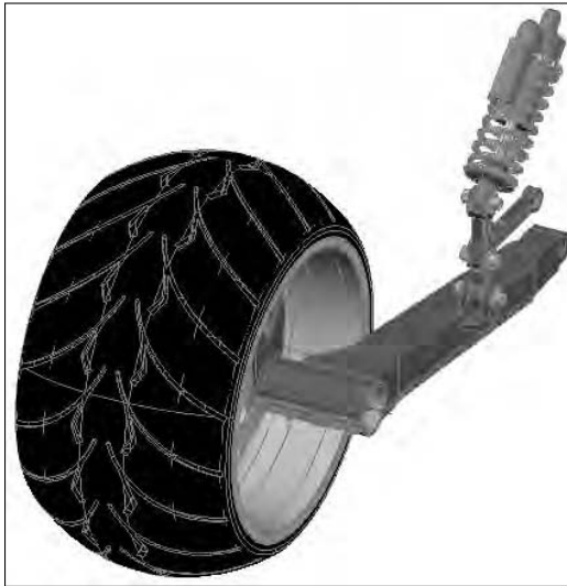
Figure 15-1: The rear assembly of a custom motorcycle.
