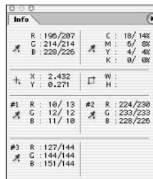
Figure 6-17: A neutral gray has close to equal amounts of red, green, and blue in it.
