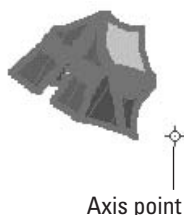
Figure 9-3: The first click creates the point of reference or axis point for the transformation.
