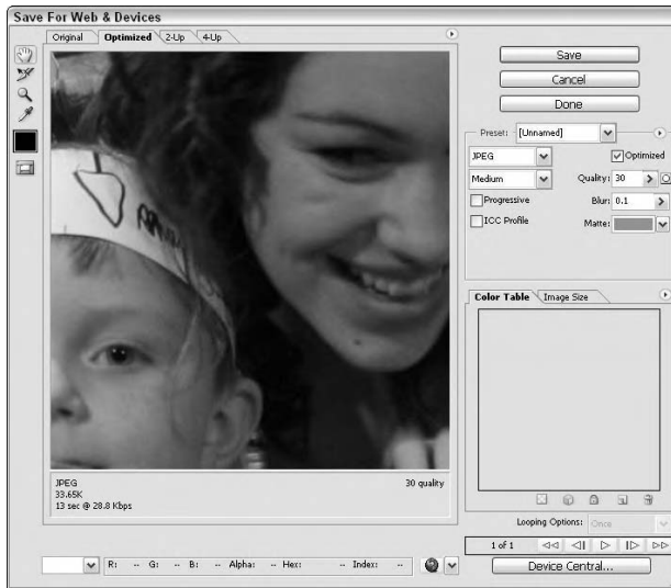
Figure 10-2: Images with smooth transitions from one color to another make good candidates for the JPEG file format.
