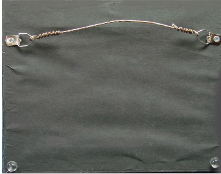
Figure 4-20: The back side of a frame has wire hanger, dust cover, and bump-on corners.
