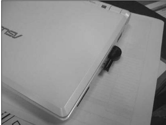
Figure 16-4: The MoGo Bluetooth adaptor (round) and the Logitech VX Nano adaptor (square) on an Eee PC.
