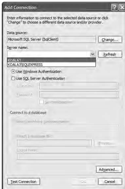
Figure 6-3: The Add Connection dialog box contains the items for specifying a connection to a database.
