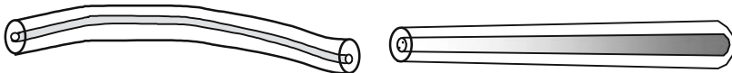
Figure 12.15. Examples of guides that are not invariant in a translation: the optogeometric properties (diameter, index of refraction, radius of curvature, . . .) vary smoothly from point to point and can be considered to remain constant along a section that is much larger than \lambda .
