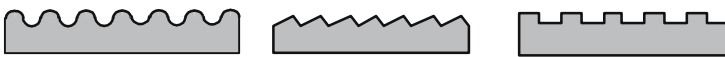
Figure 7.26. Some usual groove profiles. The periodicity ranges from 10\mu\text{m} to 0.5\mu\text{m} , i.e., 100 to 2000 grooves per millimeter.
