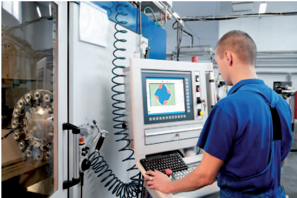
A CNC (computer numerically-controlled) milling machine cuts mechanical components out of solid steel. The software may have to solve thousands of polynomials to cut complex shapes.
