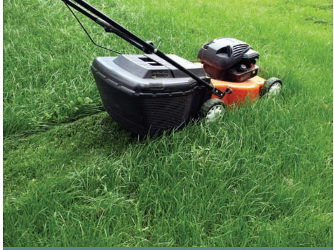
Two-stroke lawnmowers run on petrol and oil mixed in a certain ratio.
