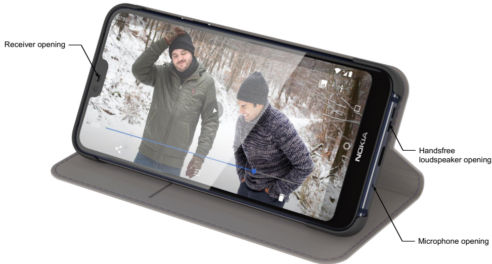
Figure 8.1 Cell phone Nokia model 7.1 showing the positions of the receiver, handsfree loudspeaker, and microphone openings. Courtesy of HMD Global OY.
