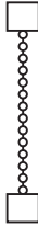
Figure 3.27 Fine mesh screen which serves as an acoustical symbol for acoustic resistance.
