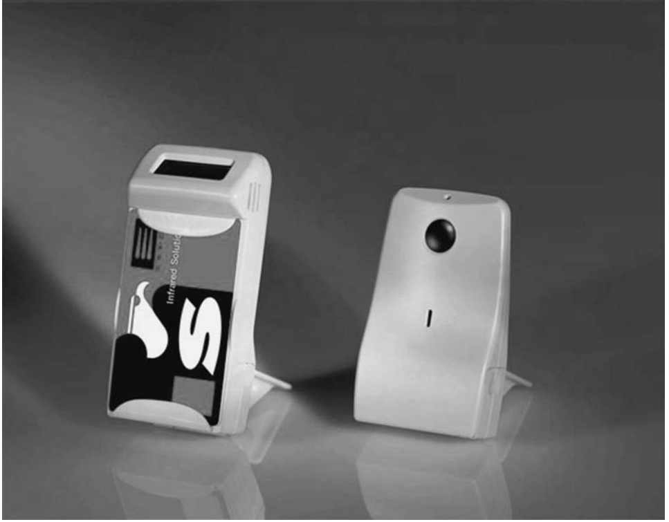
Figure 16.2 On-board unit (OBU) for road tolling (© Efkon AG)
