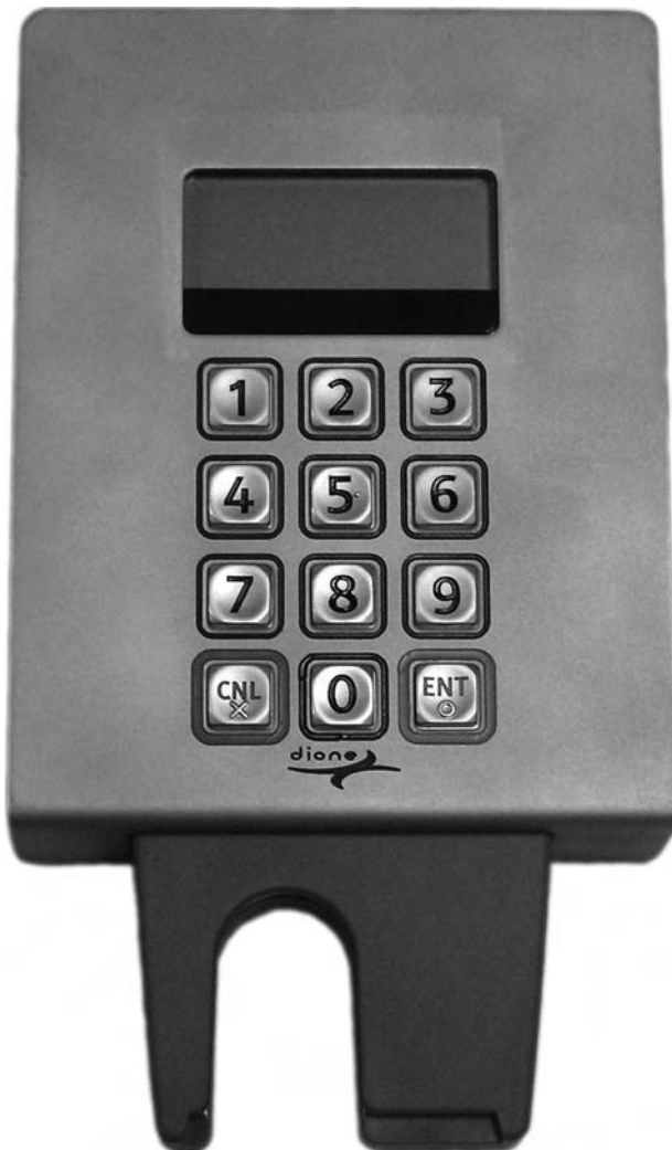
Figure 7.2 OEM card accepting device (courtesy of VeriFone Inc.)
