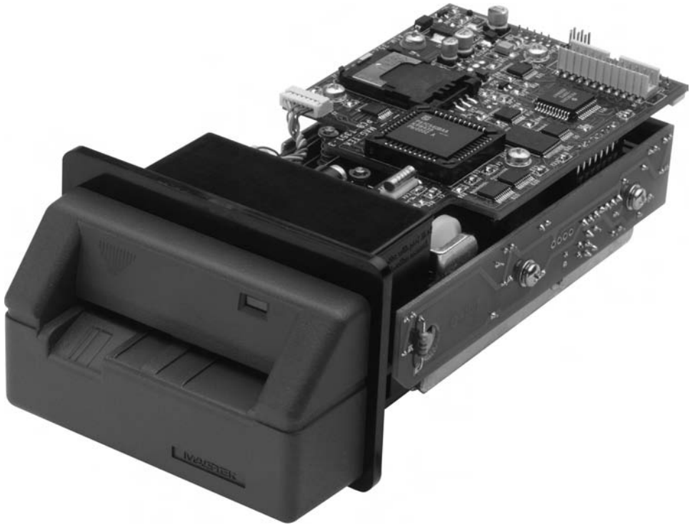
Figure 3.6 Motorised reader (© Magtek, Inc.)
